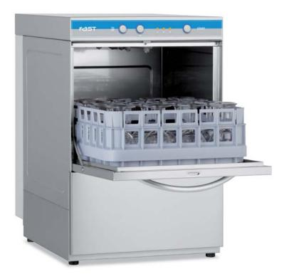
Undercounter model with 40x40 cm rack able to wash up to 750 x 7 cm diameter glasses. Useful height of 29.5 cm permits washing of up to 25.5 cm high glasses and also of up to 270 x  $\emptyset$  24 cm standard plates/hour with the specific optional support.
