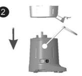
2. Place a juice bowl onto the motor block, so that juice spout pipe with the closure is found over the hollow in the appliance base unit.
