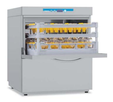
Undercounter version with 50x50 cm rack able to wash up to 1,000 wine glasses/hour. Useful height of 29 cm permits washing of up to 25.5 cm high glasses and also of up to 720 x ø 24 cm standard plates/hour. External dimensions of 60x60 cm with height limited to 72 cm permit seamless integration to replace old machines with 40x40 cm rack.
