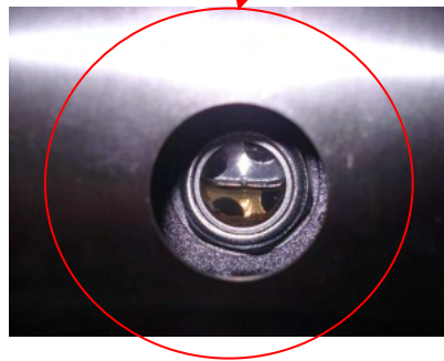
Illustration 1. Rear display for checking the oil level
