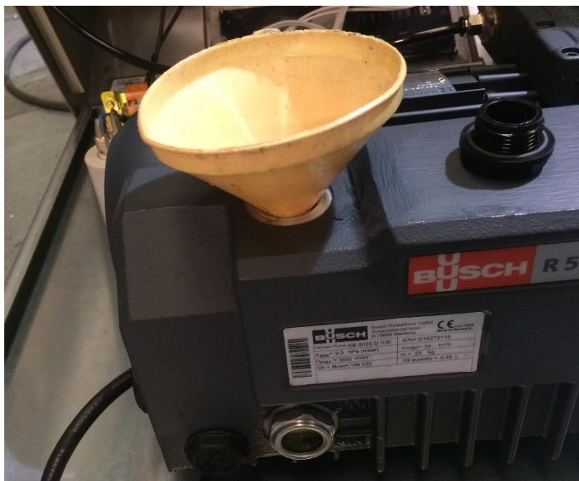
Illustration 7. Remove the oil filling plug and refill with new oil
