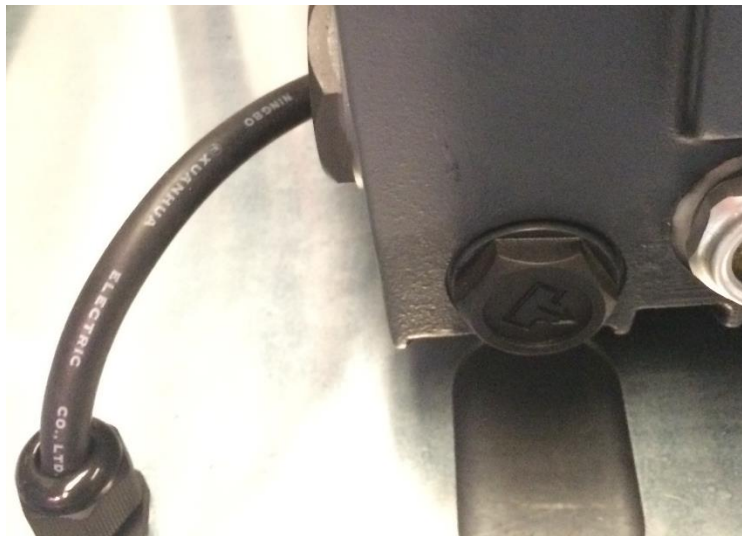
Illustration 5. Remove the oil drainage plug
