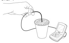
Turn the ChefAlarm on and immerse the probe into the ice bath and gently stir. When the temperature is stable and constant, note the final reading. It should be close to 0  $^{\circ}$ C. However, it may be low or high by several tenths of a degree or even one or two whole degrees. If, for example, the reading is -0.3  $^{\circ}$ C, then you are reading low by 0.3  $^{\circ}$ C.
