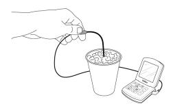
Repeat the ice bath test in Step 1. You should be spot-on or within ±0.05 °C.
