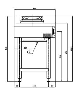
A : Gas Valve Burner G : Gas Connection
