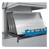
Hood version with 22-plate 50x60 cm plastic rack; optional 24-plate 61x50 cm wire rack. Maximum theoretical productivity is 1,100 and 1,200 plates/hour respectively. Useful height of 46.5 cm.
