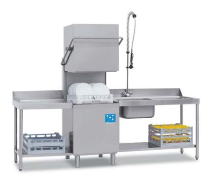
Hood version with 18-plate 50x50~cm rack also able to wash the 22-plate 54x54~cm rack (optional); maximum productivity is 720 and 880 plates/h respectively. Useful height of 40 cm.
