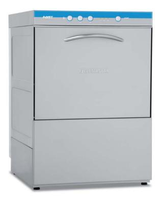
Undercounter version with 18-plate 50x50 cm rack. Maximum productivity is 720 plates/h. Useful height of 36.5 cm, can wash up to 32.5 cm high glasses. External dimensions of 57.5x60.5 cm with height limited to 82 cm permit seamless integration. Available in single-phase (FAST 160-2) or three-phase (FAST 161-2) version.
